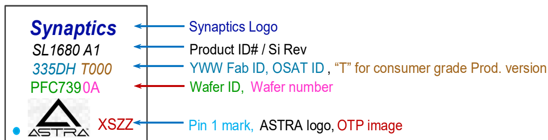
Figure 22. Package Marking and Pin 1 Location
